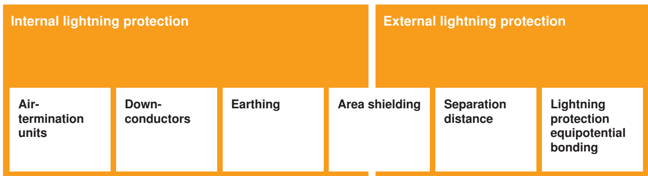
External and internal lightning protection systems
